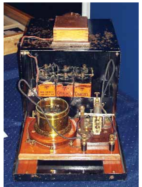
The original portable coherer receiver used by Marconi to demonstrate his invention to the public at the Toynbee Hall, London, 12 December 1896.
